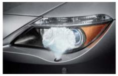
■ Headlight cleaning system helps keep lights clean of ice, mud, road salt and other coatings for maximum road illumination and enhanced driving safety.
