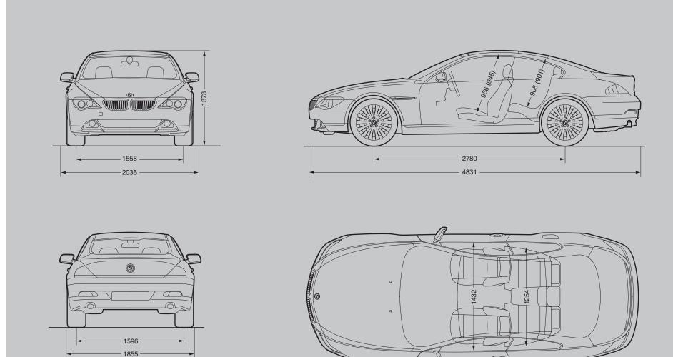
All dimensions in the technical drawings are given in millimetres. Luggage compartment volume approx. 450 litres (VDA measurement). () Measurement with glass roof.
