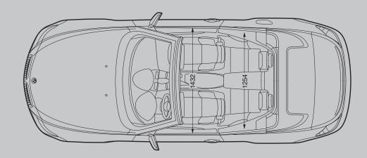
All dimensions in the technical drawings are given in millimetres. Luggage compartment volume approx. 300 litres. (350 litres with raised softtop compartment, VDA measurement.)
