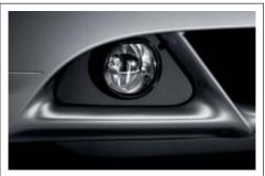
■ Foglights integrated in the front air dam provide extra safety in bad weather and situations of poor visibility. Ellipsoid free-form technology ensures a very homogeneous spread of light on to the road.
