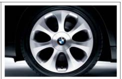
□ **Ellipsoid alloy wheels** - Style 121, 19 x 8.5 front, 245/40R-19, 19 x 9.0 rear, 275/35R-19.
