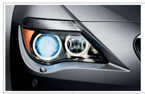
■ Xenon headlights for low and high beam, with automatic headlight range control. The sophisticated light system ensures much better illumination of the road ahead and to the side. The ellipsoid light technology offers a very high standard of light intensity and a very smooth, consistent spread of light on the road.
