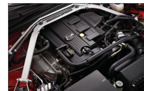
● Strut Tower Bar Adds to the structural integrity of the vehicle. Made of lightweight aluminum. Strut Tower Bar . . . . . QNCA-56-490
