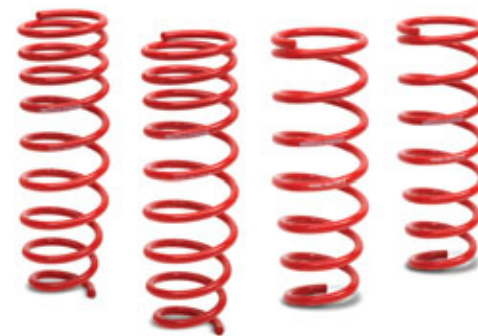
■ Sport Springs Reduce ride height by 22mm – 39mm depending on vehicle. Increases spring rates 30% over OE, resulting in enhanced steering and improved cornering. I4 Sedan Only (non-Turbo) . . . GRMS-8M-H13 V6 Sedan Only . . . . . GRMS-8M-H14 Sport and Wagon . . . . . GRMS-8M-H15
