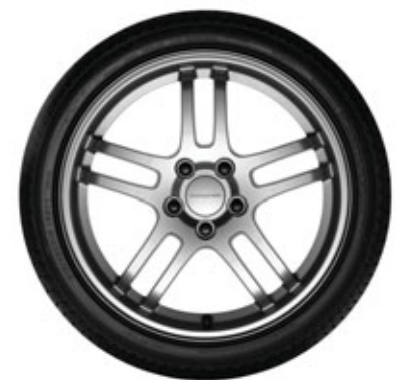
● Forged Aluminum Wheel Lightweight and strong, this forged aluminum 18x7.5J wheel is a one-piece design and weighs in at only 7.7kg. Includes centre cap and lug nuts. Recommended tire size is 215/45R18. Forged Aluminum Wheel . . . . . BLMS-8M-Z01
