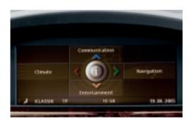
□ Navigation System Professional, including DVD drive and iDrive Controller. Destination input via voice control. Directions are given via arrows and a map displayed on an 8.8" monitor.
