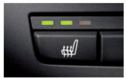
■ Seat heating for driver and front passenger (three settings): seat surface, sides and backrest are heated and quickly radiate comfortable warmth. (Optional on the BMW 323i.)
