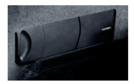
☐ **6-disc CD changer,** with MP3 decoder, located on the left-hand side of the luggage compartment.
