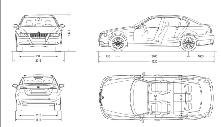
All dimensions in millimetres. Luggage compartment capacity (as per VDA standard): 460 litres on the BMW 323i and 328i/xi, 450 litres on the BMW 335i.
