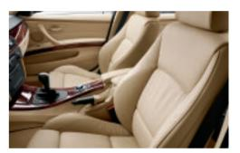
□ Sport seats for driver and front passenger (shown here in optional Beige Dakota Leather). Optimum lateral support is ensured by continuously variable electric backrest width adjustment. Seat height, backrest and seat angle, as well as thigh support, are manually adjustable.a
