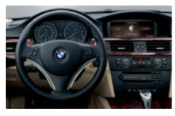
□ Leather sport steering wheel: 3-spokes, including handbrake lever handle finished in leather. Multi-function buttons for frequently used controls. (Standard on the BMW 335i.)
