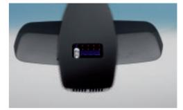
■ Rain sensor with automatic headlights. Once activated, the rain sensor will automatically switch on the windshield wipers when it begins to rain, adjusting the wiper frequency in line with rainfall intensity. The integrated automatic headlight control will switch on the low beam automatically at dusk and in tunnels.
