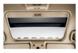
☐ Glass sunroof, electric, with wind deflector and comfort opening function via the car's remote control unit; includes reading lights at the front and illuminated vanity mirrors. (Standard on the BMW 335i.)
