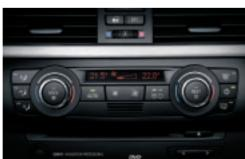
■ Automatic Air Conditioning, including AAR, micro filter, fogging and solar sensors and residual heat button, rapidly provides and maintains the selected temperature. With individual temperature control at the front (left/right) and climatized storage compartment in the centre console, including rear air vent and air conditioning. (Available only on the BMW 328i/xi and 335i.)
