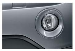
■ Foglights integrated in the front air dam ensure extra safety in bad weather and in poor visibility.
