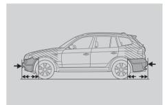
■ Bumpers with regenerating aluminum impact absorbers at the front (steel at the rear) absorb impacts without damage at speeds of up to 4 km/h; special deformation zones at the front and rear absorb impacts at up to 15 km/h without any damage to the body.
