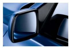
■ Exterior mirrors in body colour are electrically adjustable and heated. □ Exterior mirrors with auto-dimming function and power folding function. Both mirrors automatically dim when exposed to more than a given light intensity from following cars. (Available only on the BMW X3 3.0si.)
