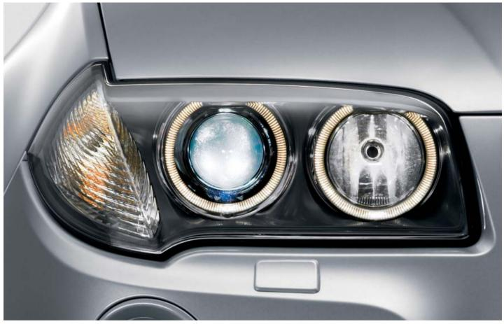
□ Xenon headlights for low and high beam, with luminous rings and automatic headlight range control, provide much better illumination of the road ahead at night or in poor visibility. These headlights also feature auto-levelling to adjust for varying passenger and cargo loads. (Standard on the BMW X3 3.0si.)
