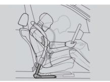
■ BMW restraint system for the driver and front passenger consists of a combination of the three-point seat belt, belt latch tensioner and belt force governor; for optimum restraint in a collision.
