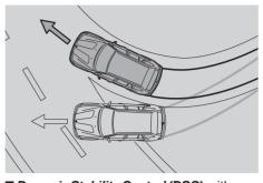
■ Dynamic Stability Control (DSC) with additional functions, including ADB-X, DTC, DBC and HDC: DSC can detect any risk of swerving early on and stabilizes the car within fractions of a second. The traction mode sub-function (DTC) allows increased wheel slip, to optimize forward thrust in any driving situation and to facilitate more nimble driving.
