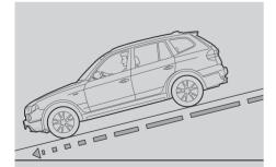
■ Hill Descent Control (HDC) enables your BMW to take even steep descents safely and reliably, automatically reducing the velocity of the car to walking speed without the driver's having to brake. As an option, HDC can also be controlled via buttons on the multi-function steering wheel.
