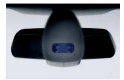
■ Rain sensor with automatic headlights. Once activated, the rain sensor will automatically switch on the windshield wipers when it begins to rain, adjusting the wiper frequency in line with rainfall intensity. The integrated automatic headlight control will switch on the low beam automatically at dusk and in tunnels.
