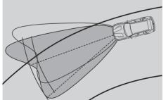
□ Adaptive Headlights system consists of electromechanically operated Xenon headlights, which swivel from side to side and thus optimally illuminate a bend the second the driver steers into it – for increased safety when driving at night or when visibility is poor. Sensors register current bend angle, yaw rate and vehicle speed. The headlights then adapt automatically to the determined bend conditions (available only on the BMW X3 3.0si).
