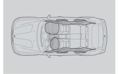
■ Airbags and all other safety components are perfectly matched to one another, meaning that in a collision only the airbag actually required is activated. Six airbags offer superior safety on demand: driver and front passenger airbags, front-to-rear head airbags and side airbags in the front (rear special order).
