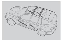
■ Door reinforcements offer optimum occupant protection in a side collision. Safety bars (reinforcement profiles) are built into the doors – for supreme door stiffness.
