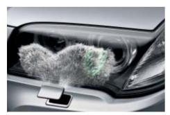
□ Headlight cleaning system ensures optimal headlight brightness in all weather conditions. The headlights are automatically cleaned in parallel with the windshield when the lights are on.
