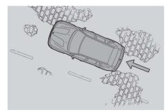
■ Automatic Differential Brake (ADB-X) emulates the function of a differential lock by means of direct intervention on a specific wheel. As soon as a wheel is about to go into a spin, ADB-X brakes it automatically until it regains traction and propulsion. With DSC active, ADB-X is supplemented by a regulation of engine performance; without DSC the function is set for maximum acceleration.
