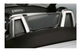
☐ The wind deflector reduces drafts and isolated turbulence in the shoulder and neck region; consists of two panes securely fitted into the roll bars and a frame-based net spanning between them. If the net is not required, it can be stored in a special storage rack in the luggage compartment.
