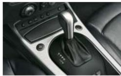
☐ Six-speed automatic gearbox with Steptronic<sup>®</sup>. Steptronic enables you to select gears manually. via the steering wheel-mounted shift paddles.
