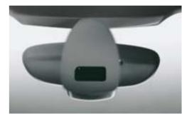
■ Rain sensor with automatic headlights uses an infrared light to measure the amount of rain. When the wipers are in the intermittent mode, the rain sensor automatically adjusts the windshield wiping interval as needed.
