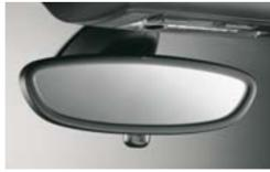
☐ Auto-dimming mirrors increase your driving safety and comfort at night. Depending on the glare intensity, the interior and exterior mirrors dim accordingly in order to minimize glare. When glare has ceased, the mirrors return to the original degree of reflection.
