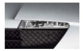
■ Foglights integrated into the front air dam. The foglights provide extra safety in bad weather conditions.
