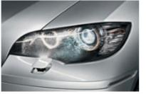
□ **High-Pressure Headlight Cleaning System** provides optimal illumination of the road ahead in all weather conditions. Headlights are automatically cleaned in parallel with the windshield when the lights are on.
