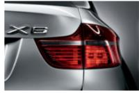
Adaptive Brakelights, two-stage, make it easier for drivers following from behind to see how hard you are applying the brakes. If you are applying the brakes in an emergency, the brakelights cover a larger area, allowing following traffic to distinguish between full application of the brakes and just a slight "tap" on the brakes. The result, clearly, is an even higher standard of driving safety on the road.
