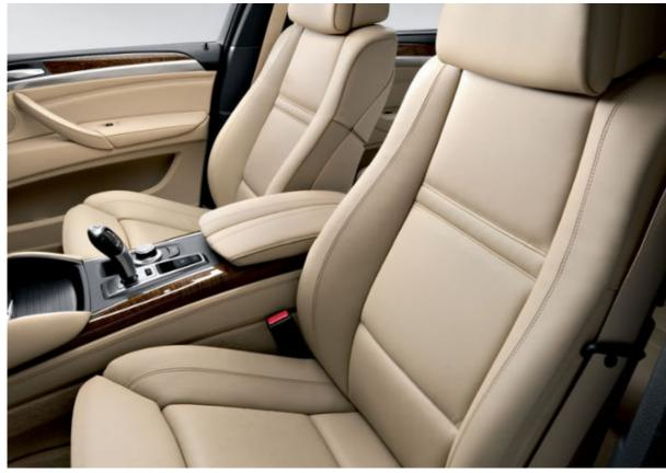
□ **Comfort Seats** for driver and front passenger, with electrical seat adjustment for all seat levels. In addition to the standard electric seat functions, Comfort Seats also provide electrically adjustable shoulder and thigh supports and backrest with lumbar support, plus two-way manual lateral adjustment for the front headrests and passenger-side memory settings.
