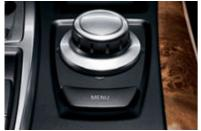
■ Controller is the central iDrive input element (for driver and passenger). Additional functions can be activated from the control display using this rotary/push button. Menu navigation is oriented to the four cardinal points. Different menus are available: Climate, Communication, Navigation, Entertainment, and on-board information.
