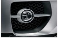
■ Foglights, integrated in the front air dam, ensure extra safety in poor visibility. Cornering lights are incorporated into the foglights, providing illumination at an angle of up to 90° to the vehicle when cornering. This allows pedestrians and cyclists to be better seen.
