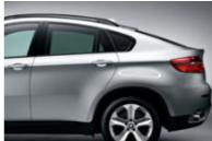
Privacy Glass for the rear side windows (behind the B-pillar) and rear window. These tinted windows reduce sun glare and ensure a pleasant temperature inside the car, even in hot weather.
