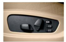
■ Seat adjustment, electric, for driver and front passenger, with memory function for driver's seat, steering column, and exterior mirrors.
