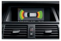
■ Park Distance Control (PDC), front and rear, makes parking easier in the narrowest spaces. The distance between the vehicle and the nearest obstacle is signalled acoustically, as well as visually in the Control Display.
