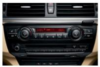
■ Automatic Climate Control, 2-zone, including Automatic Air Recirculation (AAR) with circulation filter, sun and condensation filters, and automatic temperature control (separate for driver and passenger), as well as air volume control.
