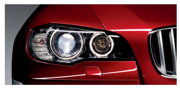
■ Xenon headlights, for low and high beam, including automatic headlight range control, for much better illumination of the road ahead in bad weather, at night, or in poor visibility. The corona rings also function as daytime driving lights, ensuring not only safety but a striking appearance at any time of day.
