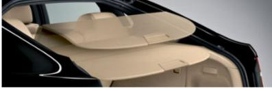
**Luggage compartment cover,** folding, can be removed easily and stowed away practically under the luggage compartment floor.
