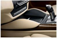
■ Knee pads, for driver and front passenger, ensure greater comfort and lateral support – especially when cornering at speed.
