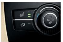
Seat heating for driver and front passenger: seat surfaces and backrests with heating in three stages for pleasant temperatures shortly after setting off.
