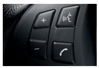
□ Voice recognition system, for adjusting e.g., navigation routes while driving. Functions are shown on the Control Display at the same time (this feature is included in the optional Technology Package and is standard on the BMW X6 xDrive50i).
