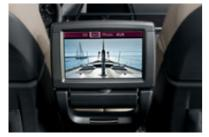
□ Rear DVD Entertainment System offers an independently controllable DVD player with a fold-down 8-inch screen. The system can be operated by wireless remote control, and features sockets for two headphones, an interface for an infrared headset, and an additional AUX/IN connection for external video sources (e.g., video camera).
