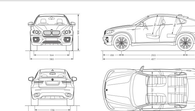
All dimensions of the technical drawings in millimetres. Luggage compartment capacity (VDA method) 570 -1,450 litres.
