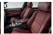
■ Sport seats for driver and passenger; highly contoured seat sides for optimal lateral support at all times. Seat height, seat angle, and backrest angle are electrically adjustable; thigh support is manually adjustable.
