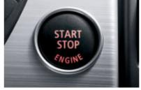
**Start/Stop button** for starting the engine. After inserting the ignition key you can start or stop the engine by pressing the button.
