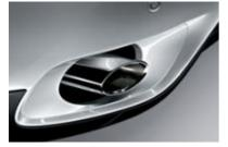
■ Tailpipes: The BMW X6 xDrive35i features two circular stainless steel tailpipes with a chrome surround.
