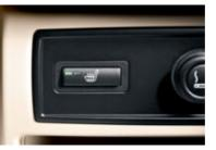
□ Seat heating at the rear, with two stages.
