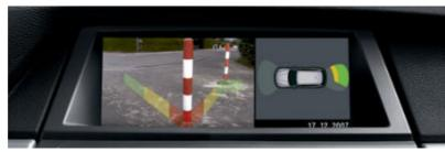
□ **Rear-view Camera** clearly shows the area behind the vehicle on the Control Display, where interactive road line markings show, for example, whether the target parking space is large enough for the vehicle. The Rear-view Camera is activated automatically when the reverse gear is selected.
