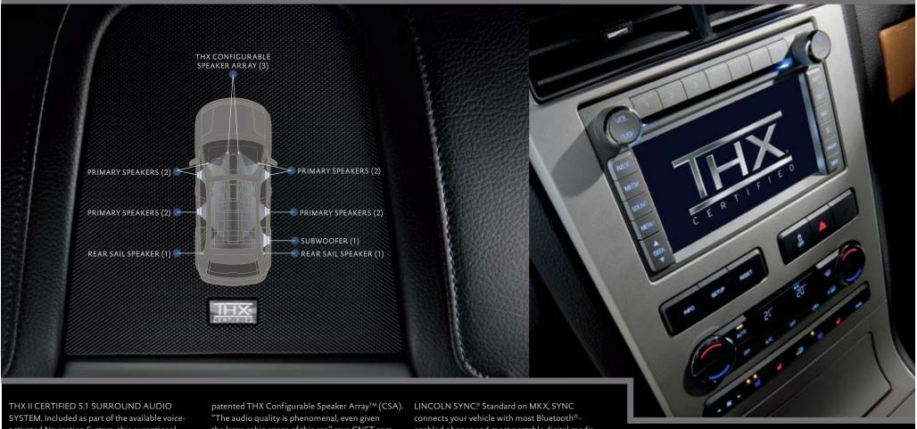
THX II CERTIFIED 5.1 SURROUND AUDIO SYSTEM. Included as part of the available voice-activated Navigation System, this exceptional audio system features 14 speakers that deliver rich, vibrant sound. A sophisticated digital signal processor provides spectral balance, wide dynamic range and superior acoustic performance. Rich, deep bass emanates from the 8-in. rear subwoofer. Power – 600 watts of it – is supplied by 12 amplifier channels. And acoustical depth pulses from the
