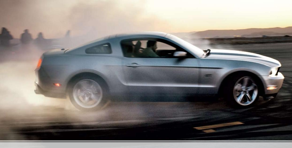
Pop the clutch and do it up. Springs, stabilizer bars and shocks were fine-tuned for a more engaging experience. Wheel/tire combos are beefier. Drag coefficient is lowered on GT and V6; also, downforce increases 23% and 37%, respectively. It all makes for one bad Mustang. Leaner and much meaner – in a really fun way, of course.
