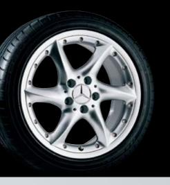
Elarneb | 6-spoke wheel, multi-piece incenio designer wheel Finish: sterling silver Wheel: 7.5 J x 17 ET 36 Tire: 225/45 R17 Option for rear axle:\* Wheel: 8.5 J x 17 ET 30 Tire: 245/40 R17 \*Not compatible with snow chains On all light-alloy wheels, use wheel bolt B6 647 0133 and the corresponding rim lock B6 647 0143 (from spring 2008: B6 647 0155).
