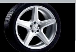
19" AMG 5-spoke wheel | Style III AMG light-alloy wheel Finish: titanium silver Wheel: 8.5 J x 19 ET 30 | Tire: 255/35 R19 Option for rear axle: Wheel: 9.5 J x 19 ET 31 | Tire: 285/30 R19 SL AMG
