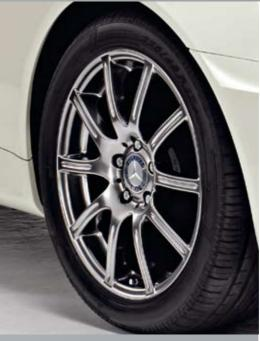
Algedi | 10-spoke wheel Finish: chrome shadow Wheel: 7.5 J x 17 ET 36 | Tire: 225/45 R17 Option for rear axle: Wheel: 8.5 J x 17 ET 30 | Tire: 245/40 R17
