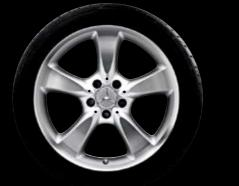
Lalande | 5-spoke wheel Finish: high-sheen Wheel: 8.5 J x 18 ET 35 | Tire: 255/40 R18 Option for rear axle: Wheel: 9.5 J x 18 ET 40 | Tire: 285/35 R18
