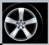
5-twin-spoke wheel Finish: titanium silver, high-sheen Wheel: 8.5 J x 18 ET 35 Tire: 255/40 R18 Option for rear axle: Wheel: 9.5 J x 18 ET 40 Tire: 285/35 R18 10-spoke wheel Finish: titanium silver or sterling silver Wheel: 8.5 J x 18 ET 35 Tire: 255/40 R18 Option for rear axle: Wheel: 9.5 J x 18 ET 40 Tire: 285/35 R18
