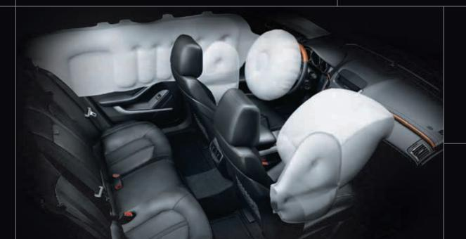
In the event of a crash, CTS is equipped to help protect you with dual frontal air bags, seat-mounted side-impact air bags and front-to-rear roof-mounted side curtain air bags.\*\*
