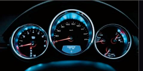
Handsome analogue gauges provide key information quickly and clearly. They're supplemented by an electronic Driver Information Centre that provides data on a variety of conditions. It even includes a tire pressure monitoring system that can inform you of tire pressure readings in real time.
