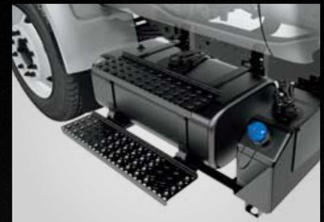
**NEW 132L FUEL TANK** and **19L DEF TANK** option mounts under the cab on the driver's side for a clean CA on Regular Cab models.
