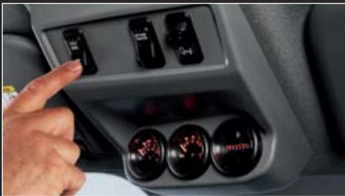
**NEW OVERHEAD GAUGE POD** places your optional gauges and auxiliary switches front and centre. Possibilities include: hour gauge, voltmeter gauge, differential lock switch, air-suspension dump switch, transmission temperature gauge, exhaust brake switch and 2-speed axle switch.
