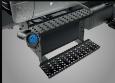
**CREW CAB 38L DEF TANK** option mounts under the cab on the passenger side.
