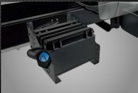
**NEW 38L DEF TANK** option mounts outside the frame rails, behind the cab on the passenger side (Regular Cab/SuperCab).
