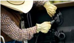
Makes connecting easy. Plug in your trailer wiring while standing upright with our class-exclusive in-bed 7-pin connector, part of the 5th-Wheel/Gooseneck Trailer Hitch Prep Package!
