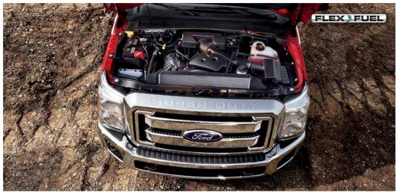
As the standard engine on F-350, the Ford built 6.2L V8 engine helps Super Duty<sup>®</sup> achieve better fuel efficiency than with the previous generation's standard 5.4L engine. It also generates best-in-class<sup>1</sup> 385 hp and 405 lb.-ft. of torque.<sup>2</sup> Rest assured that this free-breathing, E85-capable engine is ready for work. The Ford powertrain team designed, engineered, built and torture-tested it themselves. These are just some of the strengths of the 6.2L V8 powerplant:
