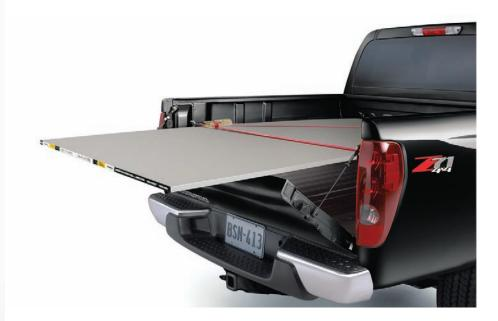
The tailgate can stop securely at a 55° angle, at the same height as the rear wheelhouses. This feature comes in very handy when you need to carry 4'x8' sheets of building material.
