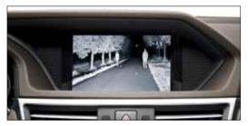
Utilizing radar technology, Night view assist provides a clear view of the road ahead when driving at night or in dark conditions.
