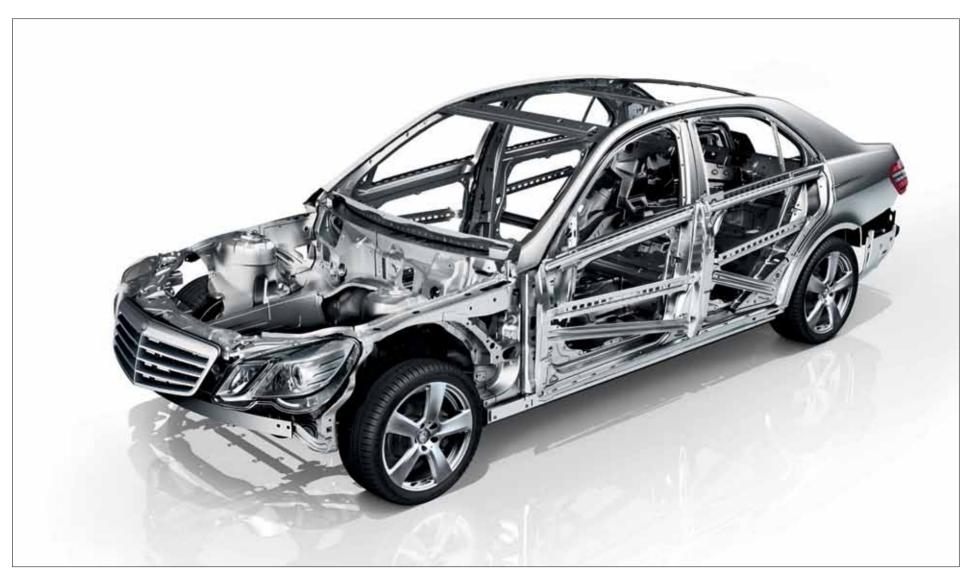
The energy-absorbing crumple zones in the front and rear sections, an extremely robust safety passenger cell, and the doors with special reinforcing elements form an effective defensive barrier in an emergency.
