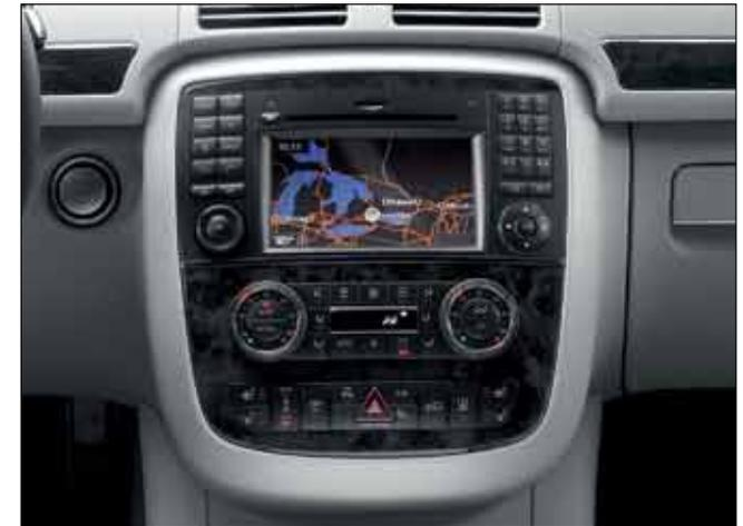
Entertainment controls are easily accessed by either the head unit or controls on the steering wheel.
