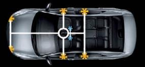
AIRBAG & SEAT-BELT SENSORS. Special onboard sensors measure the severity of a crash impact and determine whether the front seat occupants are wearing their seat belts. Within milliseconds, this information is used to determine and trigger an optimal level of airbag inflation.9
