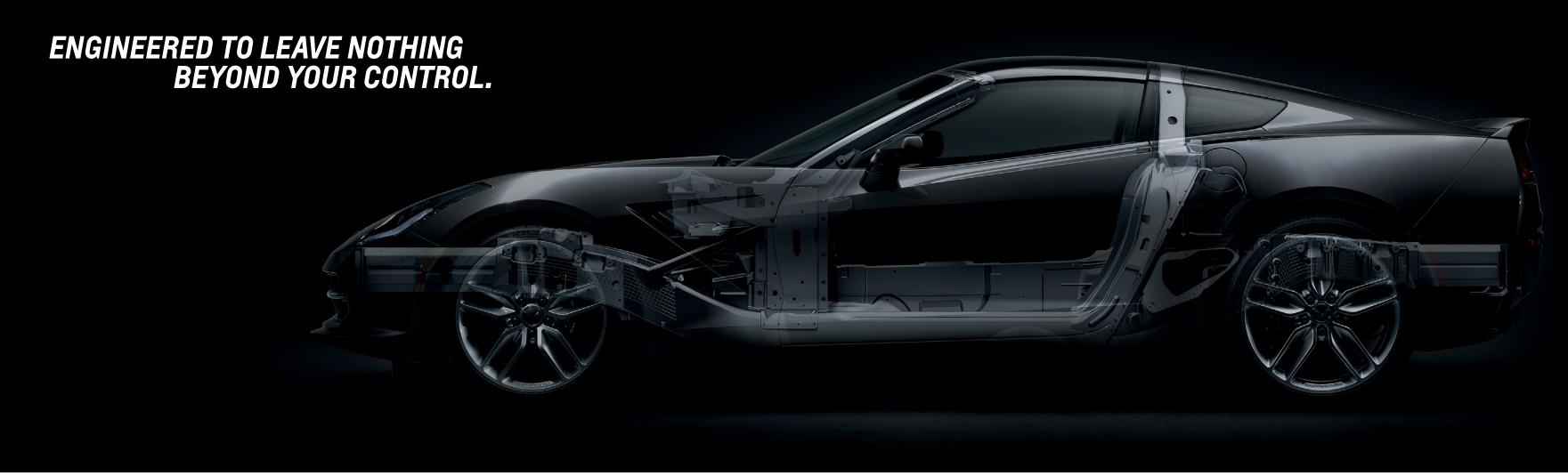
Cone-third the weight of steel, the latestgeneration Corvette aluminum space frame is 45 kilograms (100 pounds) lighter and 57% more rigid than its steel predecessor.
