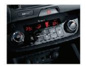
DUAL-ZONE AUTOMATIC TEMPERATURE CONTROL. Temperature control on EX and SX allows the driver and front passenger to create their own climate zones by adjusting their own temperature settings.
