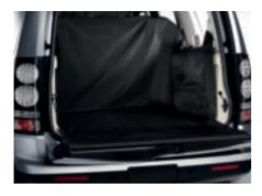
Flexible Loadspace Protector Heavy duty fabric protects loadspace up to window height. Also covers loadspace floor with second row seats folded. Includes heavy duty gloves.
