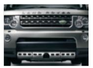
**Underbody Protection –** Non-Winch Version\*\* A sturdy aluminum undershield designed to give under-engine protection when driving in harsh off-road conditions. Winch sold separately.
