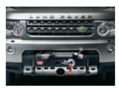
Electric Winch 4,300kg (9,500lb) maximum load capacity. Includes cover for protection when not in use. Plug-in remote control allows safe operation from up to 3.6 metres. Compatible with protection bar.
