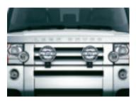
**Driving Lamp Kit\*** High performance halogen driving lamps supplied with covers. Additional mounting brackets (VPLAV0098) required.
