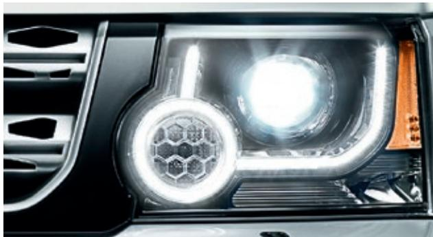
**Automatic headlights with High Beam Assist and Adaptive Xenon headlights with LED signature\*1**
