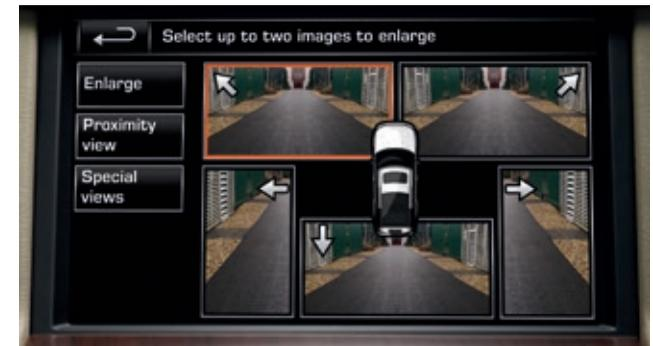
**Rear Parking Aid / Rear View Camera / Surround Camera System with the T-Junction Camera\*\***
