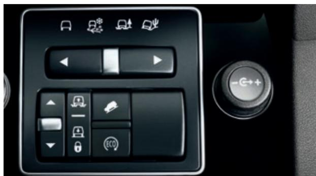
**Terrain Response System® and Gradient Release Control\*\*1**
