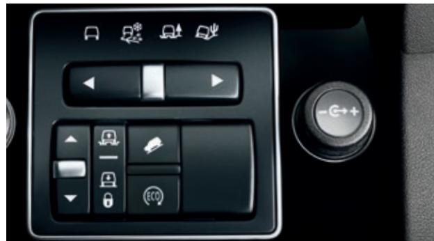
**Terrain Response System® and Gradient Release Control\*\*†**
