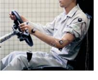
Is it possible to increase the cabin room without expanding the dimensions outside? Mazda engineers achieved this marvel by tilting the steering wheel 10 mm, increasing the head clearance by 11 mm and allowing for the seats to recline by an additional 2°. The MX-5's interior environment is designed to the utmost of form and function, because it's this attention to detail that matters when someone six feet tall takes a seat behind the wheel.
