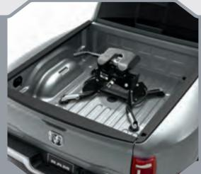
GOOSENECK/FIFTH-WHEEL varieties of towing rely on pure capabilitystarting with a strong rear structural crossmember. Note: along with the Prep Group option includes an additional 7-pin connector integrated into the rear of the bed for easier access. When the Trailer Camera Prep Group is added, the 7-pin connector is upgraded to a 7-/12-pin connector.
