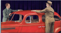
One solid sheet of equalized steel—smooth and gleaming, without a seam from end to end—forms the Ford top. Not only are the molding curves and contours more beautiful, but this new construction promises rugged strength. It binds the whole body structure into one rigid unit of steel and even more top strength is added by the reinforcing bar with 11 bars of steel on steel.
