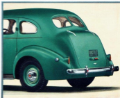
The new quarter has a new grade of wrapping beauty further enhanced by a divided top rear window of simple width and height whose safety glass pane is slanted against glare of following cars at night. The trunk is designed as an integral part of the machine and its ability creates its beauty.
