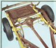
The self-control bar shown ahead of the differential adds an important part to riding comfort. Remotely from all high speeds or on rough roads, tends to steady the car itself—an objectionable effect obviated by this steady bar of spring steel.
