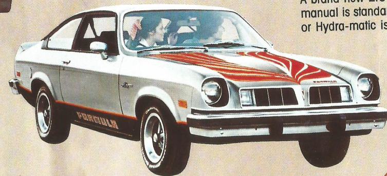
Astre New 2.5 litre-2 bbl 4 cyl. engine is standard on Formula Hatchback and Wagon. Other features include radial tires with Rally RTS suspension.
