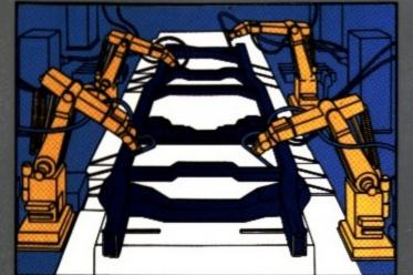
Robotic welding of the frame is fast and accurate
