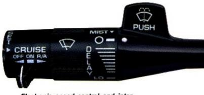
Electronic speed control and intermittent wipers are on the standard multi-function lever.
