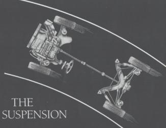
Front: Independent; struts: lower control arms with anti-dive geometry; stabilizer bar; coil springs. Rear: Independent; double wishbone design with trailing arms; stabilizer bar; coil springs.
