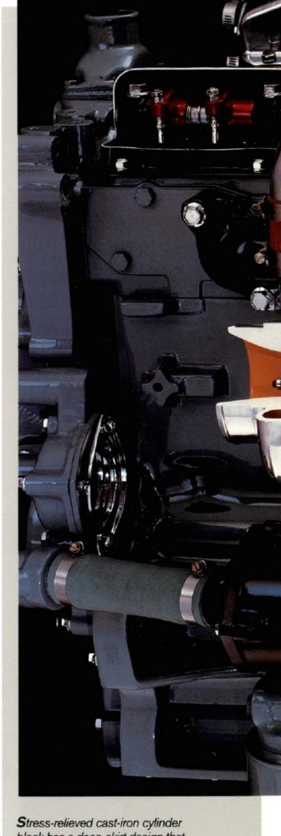
Stress-relieved cast-iron cylinder block has a deep-skirt design that extends well beneath the crankshaft to maximize rigidity and strength. Its parent bore block design actually forms a double cylinder wall compared with the single wall of wet-liner engine.
