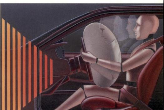
Shown here is an artist's depiction of a test of Mark VII's standard driver-side air bag Supplemental Restraint System. It inflates in less than a tenth of a second in the event of a moderate to severe frontal impact, then deflates in a fraction of a second.
