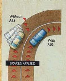
Cougar XR7's available Anti-lock Braking System (ABS) helps drivers maintain steering control during hard braking even in less-than-ideal situations. And it may be ordered with electronic Traction Assist, which helps the driving wheels grip slippery surfaces rather than spin during acceleration.
