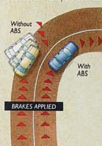
System (ABS) helps drivers maintain steering control during hard braking even in less-thanideal situations. And it includes electronic Traction Assist which helps the driving wheels grip slippery surfaces rather than spinning during acceleration.
