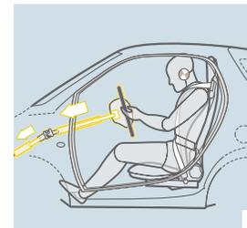
■ 2. In the event of a serious front-end collision, the steering column will retract telescopically out of harm's way.
