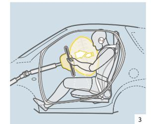
■ 3. All models are equipped with standard full-size front air bags and side air bags for enhanced protection from side impact.
