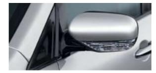
**LED turn signals** - Integrated into the side mirrors, the stylish turn signals incorporate LEDs for better visibility and enhanced safety in all lighting and weather conditions.
