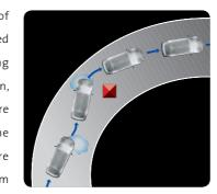
stability and traction at all times. By controlling engine output, front and rear torque distribution and brake pressure to individual wheels, VDC helps maintain stability to keep your vehicle on its intended path.
