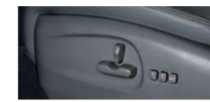
**Memory seat** - The eight-way power-adjustable driver's seat includes a memory feature that saves the precise seating preferences of two different drivers.
