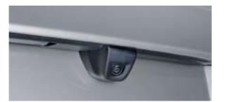
**Rear view camera** - This camera shows what's immediately behind the rear bumper on the monitor system. The monitor system also shows distance lines to help you back up safely.
