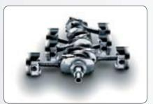
The horizontally-opposed engine, also known as the *boxer*, earned its nickname because its pistons move like a prize-fighter, alternately throwing left and right punches on a horizontal plane. The motion of the right bank of pistons counteracts that of the left bank, thereby balancing each other out and reducing engine
