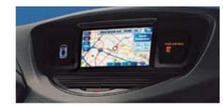
**Navigation system** - The GPS DVD-based navigation system sends map images and directions to the bright, 7-inch monitor system screen, helping you stay on track at all times.
