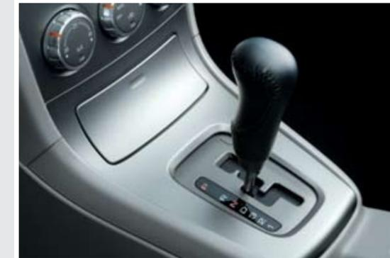
4-speed Electronic Direct Control Automatic Transmission
