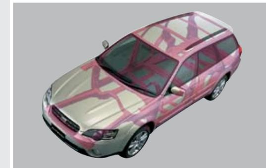
Advanced ring-shaped reinforcement frame
