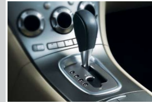
5-speed Electronic Direct Control Automatic Transmission with SPORTSHIFT™
