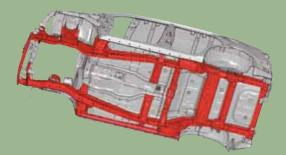
Built atop an Integrated Ladder Frame, the Grand Vitara achieves increased rigidity and durability while minimizing overall vehicle weight. The monocoque design also reduces annoying body squeaks and rattles. Additionally, this framing allows for increased ground clearance and reduced floor height, resulting in outstanding off-road capabilities. It also results in a class-leading\* towing capacity of 3000 pounds.
