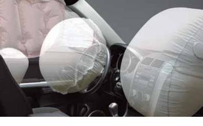
SRS dual front, seat-mounted and side curtain airbags are standard. Note: The SRS airbags are shown inflated for descriptive purposes.
