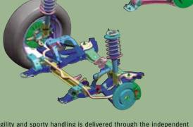
Agility and sporty handling is delivered through the independent suspension featuring front MacPherson struts and rear multi-link geometry. Both work in tandem to increase on-road responsiveness and off-road handling.
