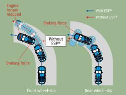
Standard on all models is the Electronic Stability Program®\* (ESP®). This advanced technology helps manage three important functions: ABS with EBD, traction control and stability control. Using various sensors, the ESP® is able to determine and hold the intended cornering line and optimize both traction and stability by reducing front and rear wheel-slip.
