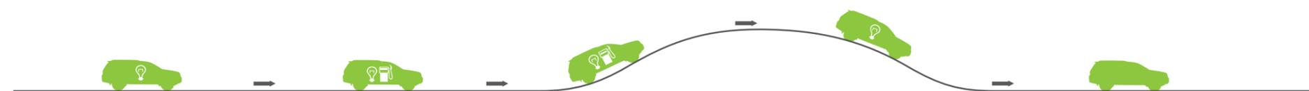
**STARTING** From initial "light" or "moderate" acceleration to low speeds, Highlander Hybrid is powered solely by a high-torque electric motor.<sup>A</sup>
