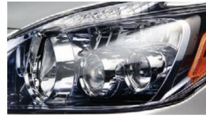
**LED LIGHTS** The available LED headlamps help reduce the electricity consumed by the headlamps approximately 20 to 30 percent, aiding the overall efficiency of Prius.
