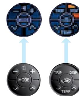
**TOUCH TRACER DISPLAY** Steering wheel-mounted controls let you adjust settings for temperature, audio mode and volume, which are conveniently displayed on the instrument panel.
