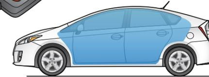
**SOLAR ROOF** The available solar roof in the 2010 Prius is embedded with solar panels. When Prius is parked in direct sunlight, these solar panels can power a fan which brings in cooler outside air, ventilating the cabin close to the ambient outside temperature.
