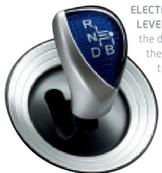
**ELECTRONIC SHIFT LEVER** Input from the driver is sent to the drive-by-wire transmission via an electronic shift lever.
