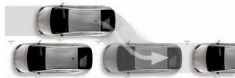
**INTELLIGENT PARKING ASSIST** Press the available Intelligent Parking Assist button and an image of the desired parking spot appears on the navigation screen, with a box indicating the final position of the vehicle. Once the driver approves the position, Prius steers and virtually drives by itself, only requiring soft braking by the driver to stop the vehicle in the intended parking spot.
