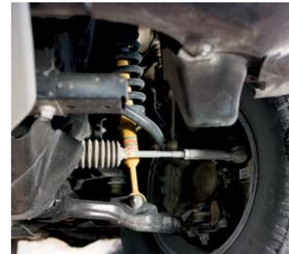
**BILSTEIN SHOCKS AND VENTILATED FRONT DISCS** Available Bilstein shocks take the edge off the bumps while the ventilated front discs help with sure stops.
