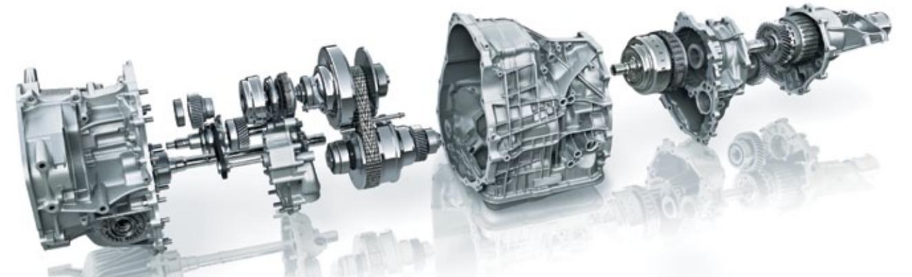
Subaru's Lineartronic® CVT (Continuously Variable Transmission) has evolved beyond traditional CVTs to become a production-car first: a CVT longitudinally paired with AWD that uses a chain instead of a belt for smooth acceleration, improved fuel efficiency and enhanced performance.
