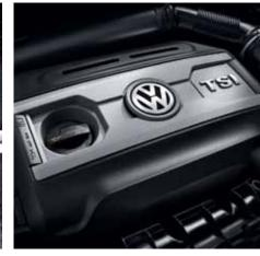
Available 2.0 TSI turbocharged engine with 200 horsepower and 2.5L engine with 170 horsepower
