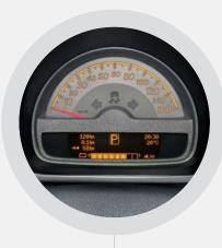
Instrument cluster with trip computer display: the multifunctional display has a READY indicator that shows when the vehicle is ready to go. It also comprises an ECO display for optimizing the driving style, a remaining range indicator, settings for departure and charging time, settings for pre-entry climate control and a service interval indicator.
