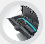
Stowage compartment in tailgate with insert for charging cable: close at hand and neatly stowed away after use, the practical tailgate compartment is a perfect fit for the charging cable. Standard for the coupé, available as an option for the cabrio.
