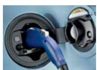
CHARGE PORT WITH ILLUMINATION The Charge Port features a Battery Charger Indicator that lets you know your battery is done charging. A built-in timer also allows you to set when the vehicle starts charging or when a full charge should be complete.
