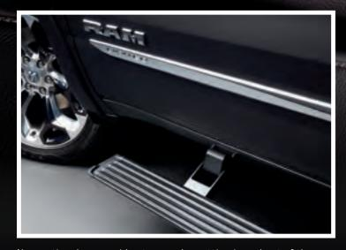
New optional power side steps make getting in and out of the cab easier than ever–and retract while driving to improve aerodynamic efficiency.
