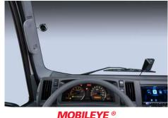
This passive safety system provides alerts and warnings for enhanced safety. The system incorporates Forward Collision Warning, Pedestrian Collision Warning, Lane Departure Warning and Headway Monitoring and Warning.
