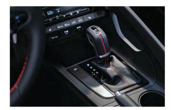
N Line: 7-speed Dual Clutch Transmission
