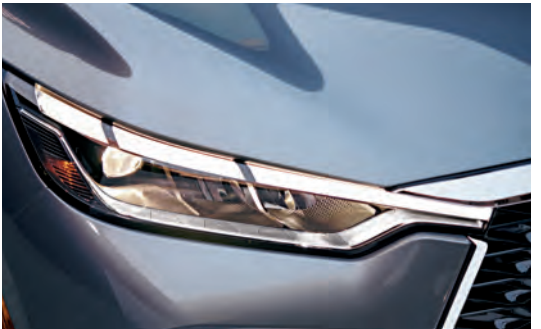
▲ DON'T JUST ILLUMINATE. SHINE. The QX60 headlights and taillights are marked by crisp segments like the keys of a piano, each lit by deep-set LEDs and a reflector that illuminate with a uniform glow rather than pinpoints of light. And with the available Vision Package, the Adaptive Front lighting System 2 can turn your low-beam headlights the direction you're steering, assuring you shine wherever you're headed.
