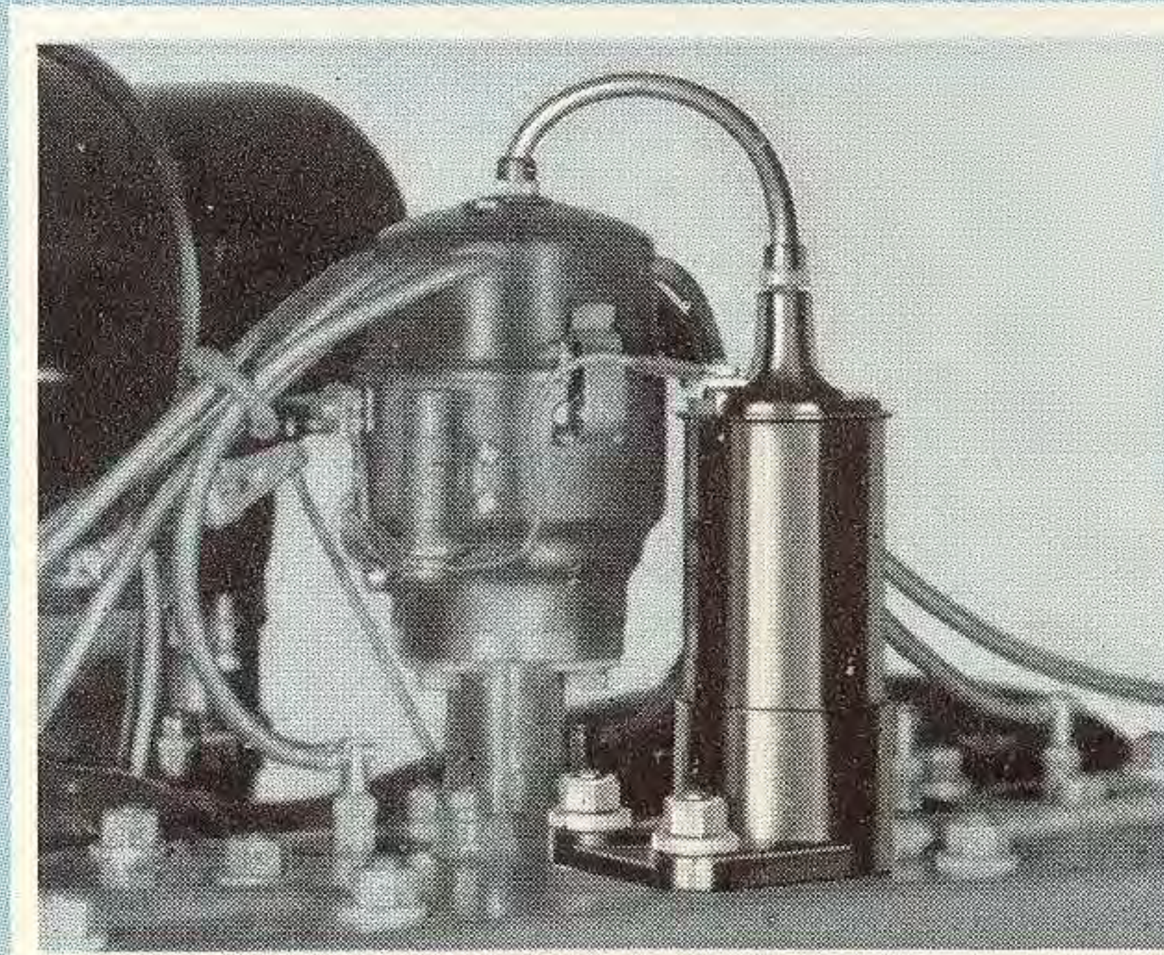
Efficient ignition is insured by a new type distributor and waterproof coil using less current
