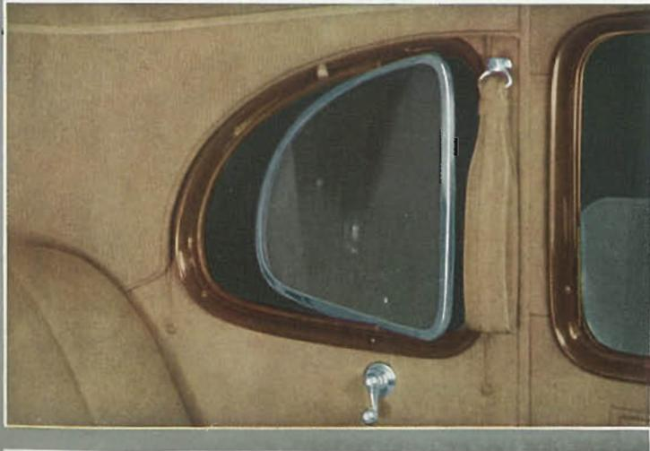
*Ventilating windows in the rear quarter grant the same adjustment for air flow to those in the rear compartment. Not only do these pivoted ventilators aid in draught control but also the scientific circulation they help create greatly increases the efficiency of any heater installation.*
